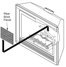
Figure 38 - Installing Brick Panels
